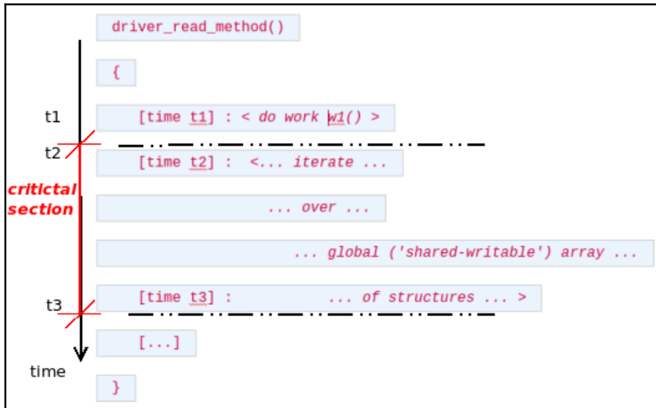
Figure 6.5 – Pseudocode – a critical section within a (fictional) driver's read method; it's wrong as there's no locking
