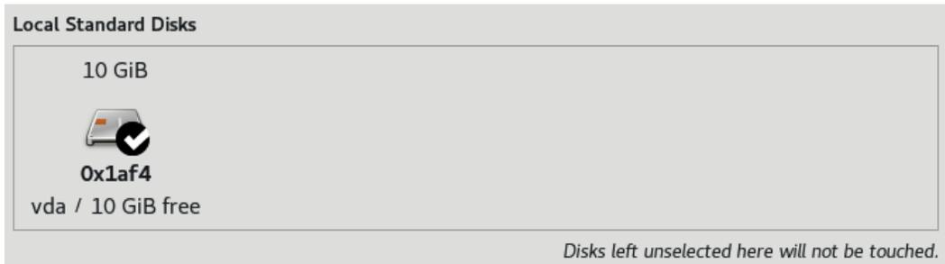
Figure 1.35 – RHEL 9 install – the INSTALLATION DESTINATION menu with a single local disk selected
