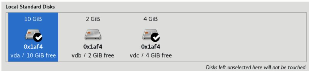
Figure 1.34 – RHEL 9 install – the INSTALLATION DESTINATION menu with several local disks selected
