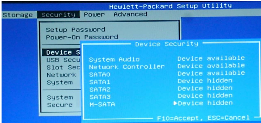
Figure 16.14: Disabling drive ports on my Hewlett-Packard Envy
