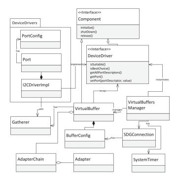
Fig. 4.5: Simplified UML diagram of the Virtual Buffers Daemon
