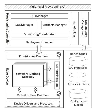
Fig. 4.2: Architecture overview of the provisioning middleware
