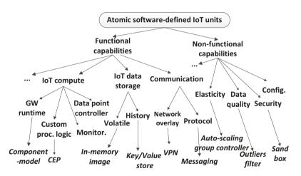
Fig. 3.5: Example classification of atomic software-defined IoT units
