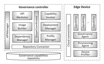
Fig. 5.4: Overview of rtGovOps architecture and deployment
