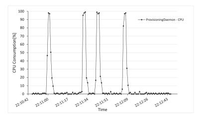
Fig. 4.10: CPU consumption of the ProvisioningDaemon
