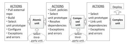
Fig. 3.6: Automated composition of software-defined IoT units
