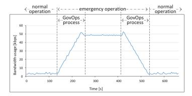
Fig. 5.8: Example execution of operational governance process in the FMS
