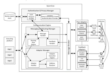
Fig. 7.3: Internal architecture of SMARTCOM middleware
