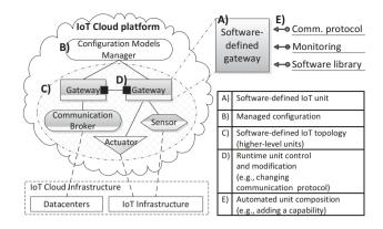
Fig. 3.2: Main enablers of software-defined IoT cloud systems
