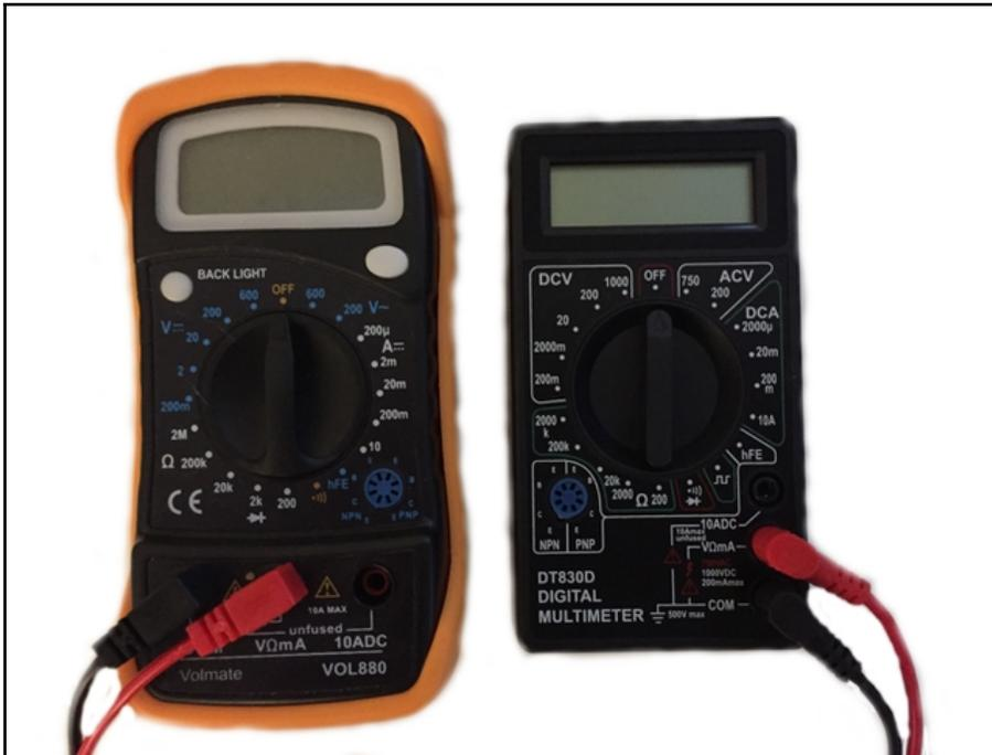
The digital multimeter has three main parts, which are the display, selection knob, and the probe ports.
