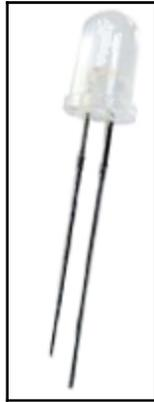
The **Light Emitting Diode** or **LED** for short, is a two-lead semiconducting device that emits light when a certain amount of current is passed through. When using a LED, we need to be very careful not to apply too much current because it is very easy to blow one. For most LED, the recommended voltage would be 5 volts.
