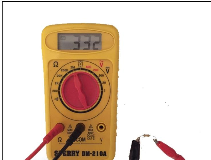
In this photograph, we are measuring a 330K Ohm resistor. If we happen to set the selection knob to low, we would overload the multimeter but almost all meters have protection, therefore, they will not be damaged by overloading them. When you overload a meter they typically show a 1 all the way to the left of the display as the following photograph shows:
