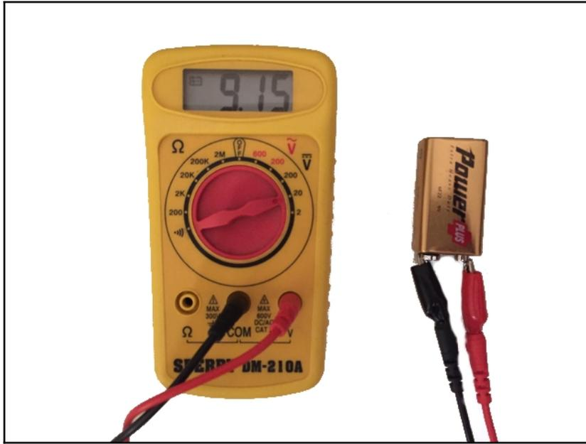
You will notice that the selector knob is set to 20V, therefore, the meter will measure up to 20V. The following photograph shows how we could measure the resistance of a resistor:
