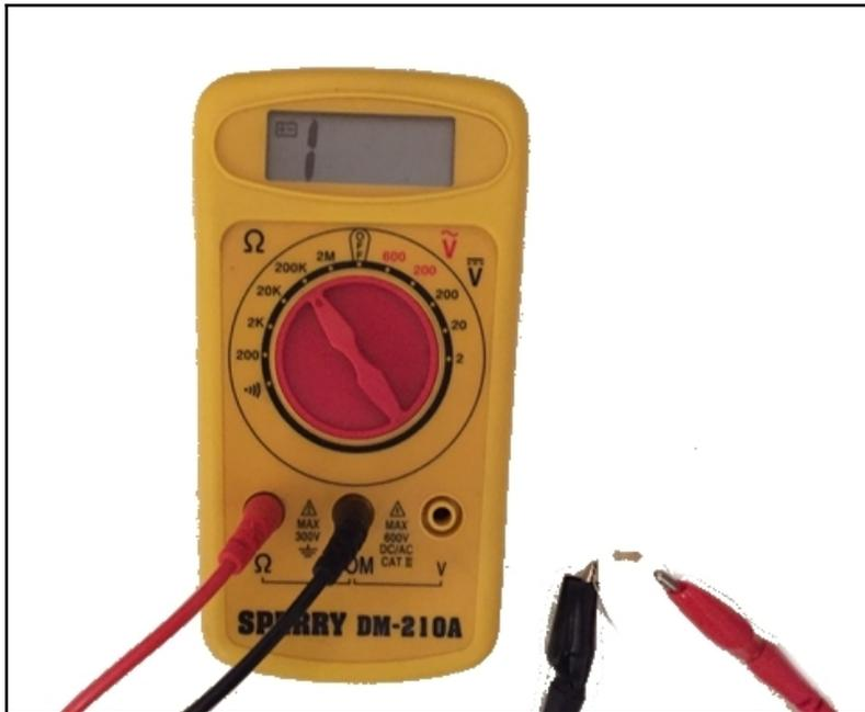
In the preceding photograph, we are trying to measure a 330K Ohm resistor with the selection knob set for a maximum of 200K Ohms. If you are not comfortable using a multimeter I would recommend searching for *multimeter video tutorials* and watching a couple videos on how to use them.
