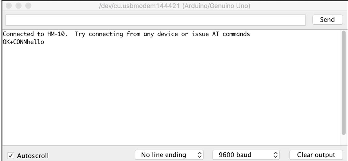
What is happening here is the message that is entered in the application is being passed from the phone application to the characteristic on the HM-10 Bluetooth module, so our application can read it. The message is sent one character at a time.
