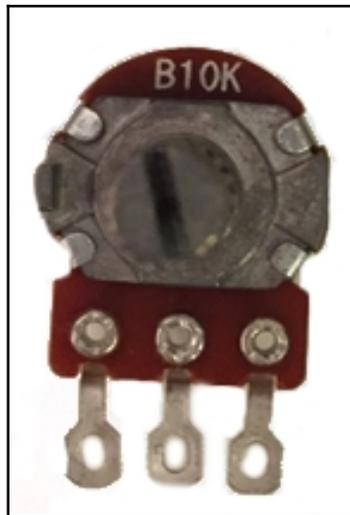
The potentiometer, also known as a pot, is a variable resistor. A potentiometer allows for the creation of a circuit where the user can change the resistance. Potentiometer comes in various shapes, sizes, and values but they all have three connectors. The resistance between the two outer connectors is fixed and is the maximum resistance of the potentiometer. The resistance between the center connector and either outer connection varies as the user turns the knob.
