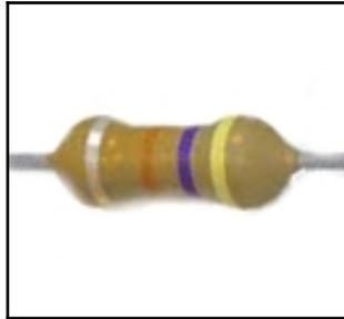
The resistor will be used in almost every circuit that we create. A resistor is an electronic component that has a specific amount of electrical resistance that never changes. The resistor limits the flow of electrons in the circuit. We will see how resistance works a little later in this chapter.
