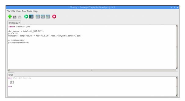
Let's take a look at the code. We will start by importing the Adafruit\_DHT library. We then create a new DHT11 object, and call it dht\_sensor. The humidity and temperature are set from the read\_retry method on the Adafruit\_DHT class.
