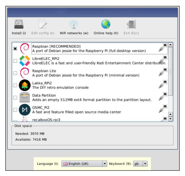
7. We will go with the top option, **Raspbian**. Check the box beside **Raspbian** [RECOMMENDED] and then click on the **Install (i)** button at the top-left corner of the dialog. Raspbian will start installing on your Raspberry Pi. You will see a progress bar with previous graphics, describing various features of the Raspbian operating system:
