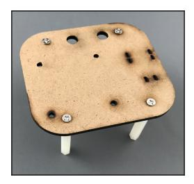
2. Screw the motor driver board (**D**) to **E** using four 10 mm M3 bolts and nuts. Refer to the following photo for the proper orientation:
