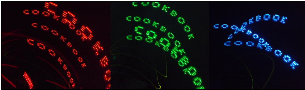
Persistence of vision using RGB LEDs
