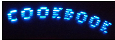
The message is displayed by the RGB LEDs - here, we are using green and blue together
