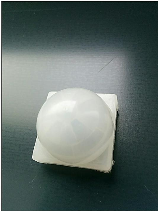
The sensor itself is located under the dome Fresnel lens and it has an infrared filter in front of it.
