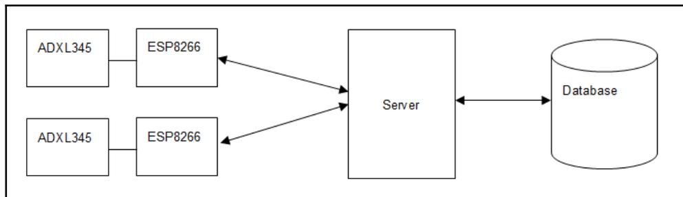
The final circuit can also include a time-series database such as InfluxDb, for storing the values transmitted by the ADXL345.
