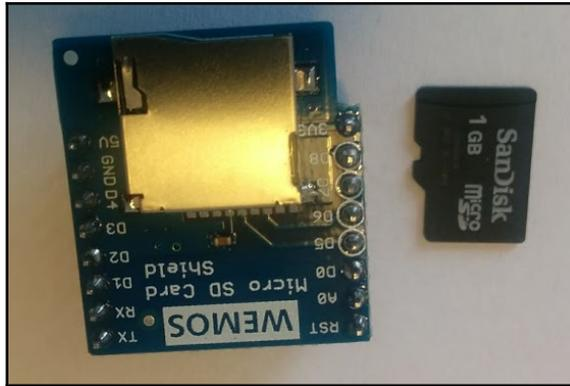
Since the microSD card is a shield for the Wemos D1 mini, it is easy to stack them; you just need to solder the pins that are coming into the package:
