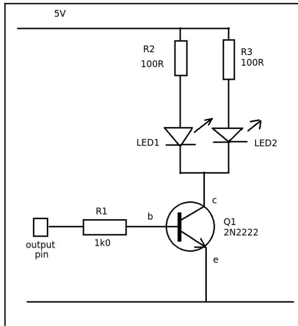
Connect the output pin to the GPIO 12 from the ESP8266 the ground to the GND pin, and 5V to 5V from your ESP.
