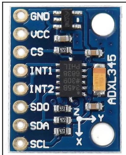
The **ADXL345** can be connected to the ESP8266 over SPI or I2C lines. In our case, we will use the I2C connection. The bus address on which the accelerometer will respond is 0x53.
