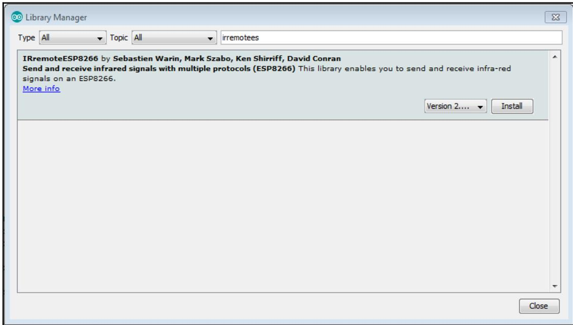
After the library is installed and the connections to the ESP are done, let's use the following code to send over an MQTT topic a command to open or close a Panasonic TV. Since the same Infrared command is used to power on or power off, you just need to receive something on the MQTT topic to send an infrared command to the TV:
