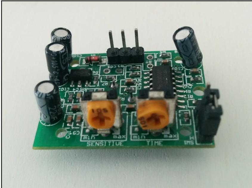
On the module there are two variable resistors that allow you to modify two things:
