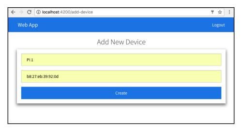
Add a new device by giving it a name. I named my device Pi 1 and added the mac address. We will use the mac address of the device as a unique way of identifying the device.
