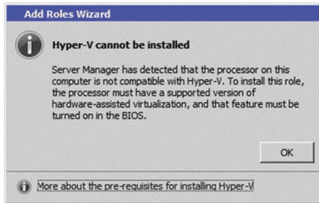
FIGURE 4.2 Warning window that Hyper-V cannot be installed
