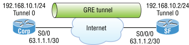
FIGURE 21.24 Example of GRE configuration
