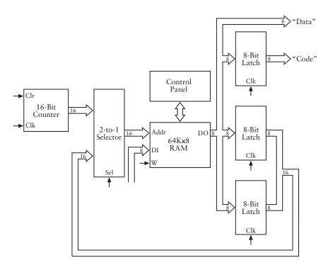
We've made a lot of progress. Now it's possible to enter the instructions and the data in a single RAM array. For example, the diagram on the next page shows how to add two 8-bit numbers together and subtract a third.
