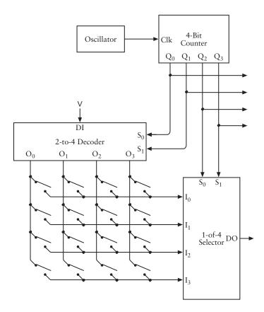
The 16 keys of the keyboard are shown as simple switches in the lower left area of this diagram. A 4-bit counter repetitively and very quickly cycles through the 16 codes corresponding to the keys. It must be fast enough to cycle through all the codes faster than a person can press and release a key.
