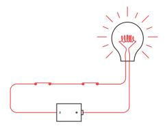
The key word here is *and*. Both the left switch *and* the right switch must be closed for the current to flow through the circuit.
