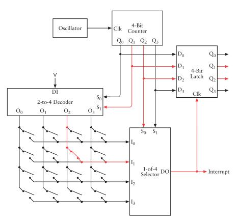
That's the code corresponding to that key. When that key is pressed, no other counter output will cause the output of the selector to be 1. Each key has its own code.
