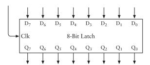
This latch is capable of saving 8 bits at once. The eight inputs on the top are labeled  $D_0$  through  $D_7$ , and the eight outputs on the bottom are labeled  $Q_0$  through  $Q_7$ . The input at the left is the Clock. The Clock signal is normally 0. When the Clock signal is 1, the 8-bit value on the D inputs is transferred to the Q outputs. When the Clock signal goes back to 0, that 8-bit value stays there until the next time the Clock signal is 1.
