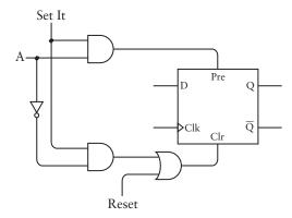
Normally the Set It signal is 0. In that case, the Preset input to the flip-flop is 0. The Clear input is also 0 unless the Reset signal is 1. This allows the flip-flop to be cleared independently of the Set It signal. When the Set It signal is 1, the Preset input will be 1 and the Clear input will be 0 if A is 1. If A is 0, the Preset input will be 0 and the Clear input will be 1. This means that Q will be set to the value of A.
