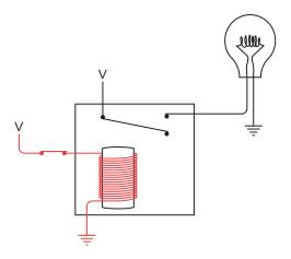
Using the terminology of switches, this type of relay is called a *double-throw* relay. It has two outputs that are electrically opposite—when one has a voltage, the other doesn't.
