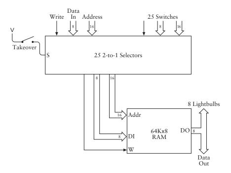
When the Takeover switch is open (as shown), the Address, Data input, and Write inputs to the  $64K \times 8$  RAM array come from external signals shown at the top left of the 2-to-1 Selectors. When the Takeover switch is closed,
