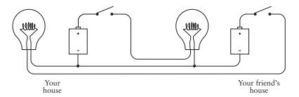
Notice that the negative terminals of the two batteries are now connected. The two circular circuits (battery to switch to bulb to battery) still operate independently, even though they're now joined like Siamese twins.
