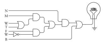
The symbols down the left side of the circuit diagram are in the same order as they appear in the expression. These signals come from the switches wired with inverters and the 2-line-to-4-line decoder. Notice the use of the inverter for the (1 - W) part of the expression.
