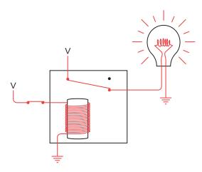
These diagrams of the relay show two voltage sources and two grounds, but in all the diagrams in this chapter, all the V's can be connected to one another and all the grounds can be connected to one another. All the networks of relays and logic gates in this chapter and the next will require only one battery, although it might need to be a big battery. For example, the preceding diagram can be redrawn with only one battery like this:
