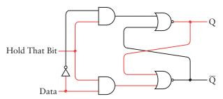
The Q output is now the same as the Data input, and  $\overline{Q}$  is the opposite. Now Hold That Bit can go back to being 0:
