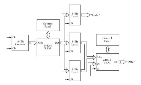
The process of retrieving an instruction from memory is known as the *instruction fetch*. In our machine, each instruction is 3 bytes in length, and it's retrieved from memory 1 byte at a time; the instruction fetch requires three cycles of the Clock signal. The entire *instruction cycle* requires a fourth cycle of the Clock signal. These changes certainly complicate the control signals.
