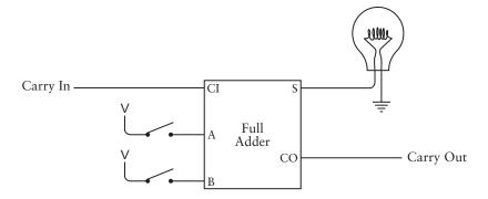
The carry output from the first Full Adder is an input to this second Full Adder. Each subsequent column of digits is wired the same way. Each carry output from one column is a carry input to the next column.
