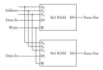
The Address and Write inputs of the two  $8 \times 1$  RAM arrays are connected, so the result is an  $8 \times 2$  RAM array:
