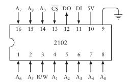
The 2102 is a member of the MOS (metal-oxide semiconductor) family of semiconductors, which is the same technology used for the 8080 and 6800 microprocessors themselves. MOS semiconductors can be easily connected to TTL chips; they generally have a higher density of transistors than TTL but aren't as fast.
