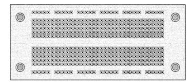
Each short row of 5 holes is electrically connected underneath the plastic base. You insert chips into the breadboard so that a chip straddles the long central groove and the pins go into the holes on either side of the groove. Each pin of the IC is then electrically connected to 4 other holes. You connect the chips with pieces of wires pushed into the other holes.
