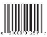
We're tempted to try to visually interpret the UPC in terms of thin bars and black bars, narrow gaps and wide gaps, and indeed, that's one way to look at it. The black bars in the UPC can have four different widths, with the thicker bars being two, three, and four times the width of the thinnest bar. Similarly, the wider gaps between the bars are two, three, and four times the width of the thinnest gap.
