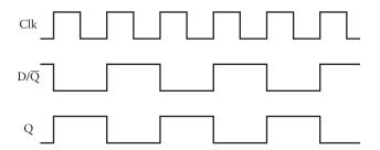
When the Clock input goes from 0 to 1, the value of D (which is the same as  $\overline{Q}$ ) is transferred to Q, thus also changing  $\overline{Q}$  and D for the next transition of the Clock input from 0 to 1.
