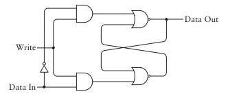
This is the same flip-flop, but now the Q output is named Data Out, and the Clock input (which started out in Chapter 14 as *Hold That Bit*) is named
