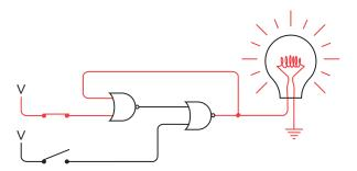
The magic occurs when you now open the upper switch. Because the output of a NOR gate is 0 if either input is 1, the output of the left NOR gate remains the same and the light remains lit:
