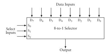
The 8-to-1 Selector has eight Data inputs (shown at the top) and three Select inputs (shown at the left). The Select inputs choose which of the Data inputs appears at the Output. For example, if the Select inputs are 000, the Output is the same as  $D_0$ . If the Select inputs are 111, the Output is the same as  $D_7$ . If the Select inputs are 101, the Output is the same as  $D_5$ . Here's the logic table:
