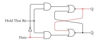
The circuit now remembers the value of Data when Hold That Bit was last 1, regardless of how Data changes. The Data signal could, for example, go back to 0 with no effect on the output:
