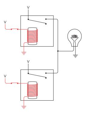
This behavior is exactly opposite that of the AND gate. This is called *NOT AND* or, more concisely, *NAND*. The NAND gate is drawn just like the AND gate but with a circle at the output, meaning the output is the inverse of the AND gate:
