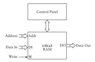
When the Takeover switch is closed, you can use the 16 Address switches to select any of 65,536 addresses. The lightbulbs show you the 8-bit value currently stored in memory at that address. You can use the 8 Data switches to define a new value, and you can write that value into memory using the Write switch.
