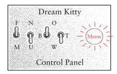
The switches are on (closed) when they're up, and off (open) when they're down. The two switches for the cat's color are labeled somewhat obscurely, I'm afraid, but that's a drawback of reducing this panel to the bare minimum: The left switch of the pair is labeled B; that means that the left switch on
