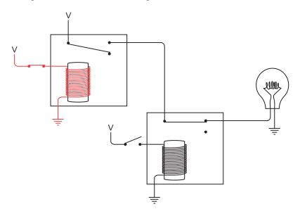
The light goes off because power is no longer being supplied to the second relay. Similarly, if the bottom switch is closed, the light is also off:
