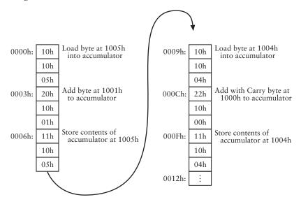
At the completion of these six instructions, the 16-bit value at memory locations 1004h and 1005h will equal A7h times 1. Therefore, these six instructions have to be repeated 27 more times in order for that 16-bit value to equal A7h times 1Ch. You can achieve this by typing in these six
