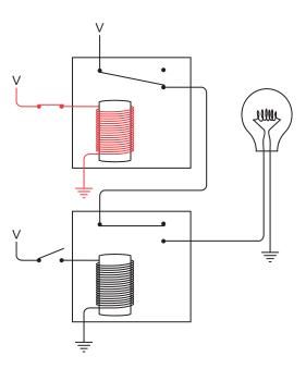
Still the lightbulb doesn't light because the bottom switch is still open and that relay isn't triggered. We can try opening the top switch and closing the bottom switch:
