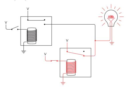
The bulb also lights if both switches are closed:
