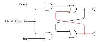
Recall that the output of an AND gate is 1 only if both inputs are 1. In this diagram, the Q output is 0 and the  $\overline{Q}$  output is 1.
