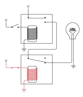
The lightbulb is still not lit. The current can't reach the lightbulb because the first relay isn't triggered. The only way to get the bulb to light up is to close both switches:
