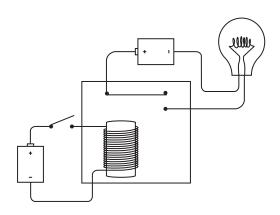
Notice that the switch at the left is open and the lightbulb is off. When you close the switch, the battery at the left causes current to flow through the many turns of wire around the iron bar. The iron bar becomes magnetic and pulls down a flexible metal contact that connects the circuit to turn on the lightbulb:
