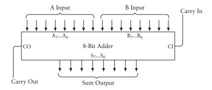
As you probably recall, the inputs A0 through A7 and B0 through B7 were connected to switches that indicated two 8-bit values to be added. The Carry In input was connected to ground. The S0 through S7 outputs were connected to eight lightbulbs that displayed the result of the addition. Because the addition could result in a 9-bit value, the Carry Out output was also connected to a ninth lightbulb.
