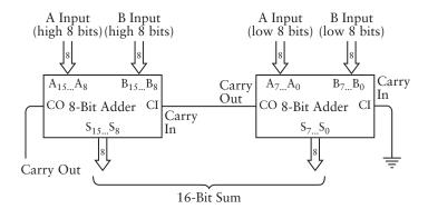
The Carry Out of the adder on the right is connected to the Carry In of the adder on the left. The adder on the left has as input the most-significant eight digits of the two numbers to be added and creates as output the most-significant eight digits of the result.
