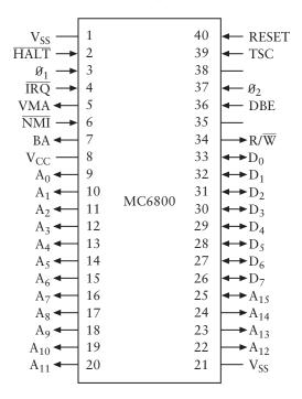
The  $V_{ss}$  indicates Ground, and  $V_{cc}$  is 5 volts. Like the 8080, the 6800 has 16 output Address signals and 8 Data signals used for both input and output. There's a RESET signal and a  $R/\overline{W}$  (read/write) signal. The  $\overline{IRQ}$  signal stands
