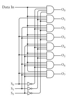
Again, notice that the inputs to the sixth AND gate from the top include  $S_0$ ,  $\bar{S}_1$ ,  $S_2$ . No other AND gate has these three inputs. So if the Select inputs are 101, then all the other AND gates will have an output of 0. The sixth AND gate from the top will possibly have an output of 0 if the Data Input is 0 or an output of 1 if the Data Input is 1. Here's the complete logic table:
