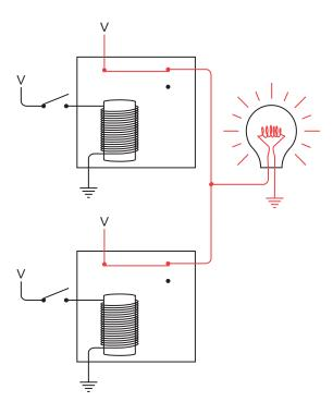
In this case, the two outputs are connected, which is similar to the OR configuration but using the other contacts. The lightbulb is on when both switches are open.
