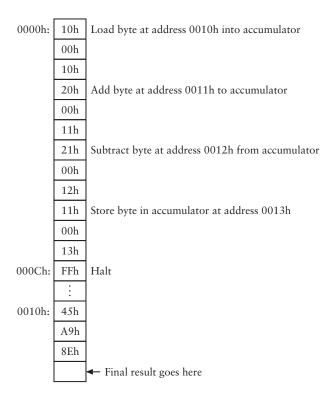
As usual, the instructions begin at 0000h because that's where the counter starts accessing the RAM array after it has been reset. The final *Halt* instruction is stored at address 000Ch. We could have stored the three numbers and the results anywhere in the RAM array (except in the first 13 bytes, of course, because those memory locations are occupied by instructions), but we chose to store the data starting at address 0010h.
