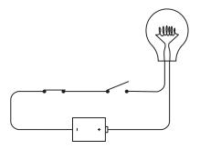
Similarly, if you leave the left switch open and close the right switch, nothing happens. The lightbulb lights up only if both the left switch and the right switch are closed, as shown on the next page.
