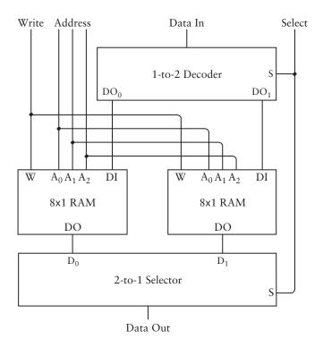
The Select input that goes to both the Decoder and the Selector essentially selects between the two  $8 \times 1$  RAM arrays. It's really a fourth address line. So this is actually a  $16 \times 1$  RAM array:
