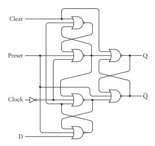
The Preset and Clear inputs override the Clock and Data inputs. Normally these two inputs are 0. When the Preset input is 1, Q becomes 1 and  $\overline{Q}$  becomes 0. When the Clear input is 1, Q becomes 0 and  $\overline{Q}$  becomes 1. (Like
