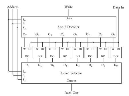
And here's the complete circuit with the 8 latches:
