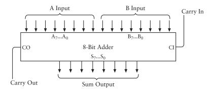
This is a common way to label the separate bits of a multibit number. The bits  $A_0$ ,  $B_0$ , and  $S_0$  are the *least-significant*, or rightmost, bits. The bits  $A_7$ ,  $B_7$ , and  $S_7$  are the *most-significant*, or leftmost, bits. For example, here's how these subscripted letters would apply to the binary number 0110-1001:
