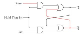
Only when the Hold That Bit signal is 1 will this circuit function the same way as the normal R-S flip-flop shown earlier:
