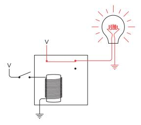
In this case, the lightbulb goes out when you close the switch. A single relay wired in this way is called an *inverter*. An inverter isn't a logic gate (logic gates always have two or more inputs), but it's often very useful nonetheless. It's represented by a special symbol that looks like this:
