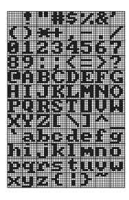
These are the characters corresponding to ASCII codes 20h through 7Fh. (No visible characters are associated with ASCII codes 00h through 1Fh.)
