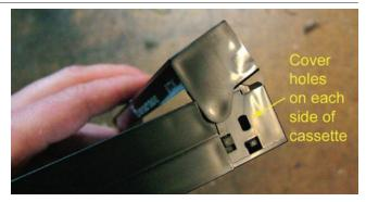
**Trick #2.** With your sacrificial videocassette partly rewound, remove its screws and reassemble it with adhesive tape. Load it into the VCR. Once it's happily loaded, unstick the tape, take the top half off, and remove the reels. If your VCR precludes you from disassembling the videocassette *in situ*, remove its windows so you can get your fingers inside.
