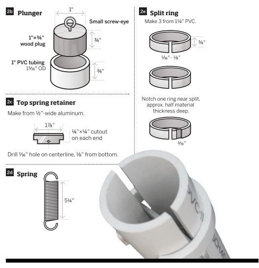
**2b.** Make the plunger from 1" PVC pipe, following the plunger diagram. Cut the 1"-diameter wood disk on a band saw, sand it to fit tightly in the ring, and glue it in place. Sand the top and bottom of the plunger flat and square, then insert a small screw eye in the center of one face.
