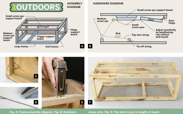
Fig. A: Frame assembly diagram. Fig. B: Hardware diagram. The latch releases the trap door when the animal takes the bait and trips the trigger string. Fig. C: To make the door lock, bend a 6" length of
