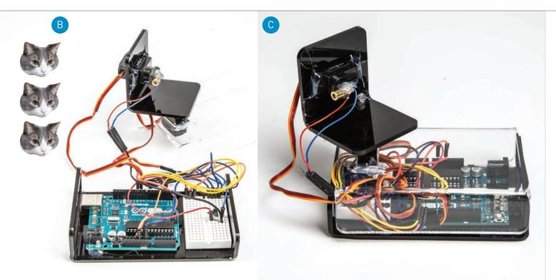
to the top of your Arduino enclosure, as shown in Figure <sup>B</sup>. Then mount the laser to the bracket as well, pointing straight ahead level. After you've gotten the system working, you'll want to tilt the laser to the floor or another surface your cats can reach.
