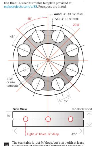
a 12" length of pipe for safe cutting on a power saw.
