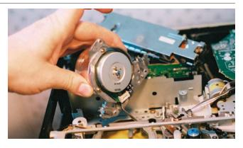
**4 DETACH THE DRUM FROM THE MOTOR.** To reduce the load on the motor, remove the actual video head drum. These are usually attached to the motor by screws on top, but you might have to unsolder connections to the heads.
