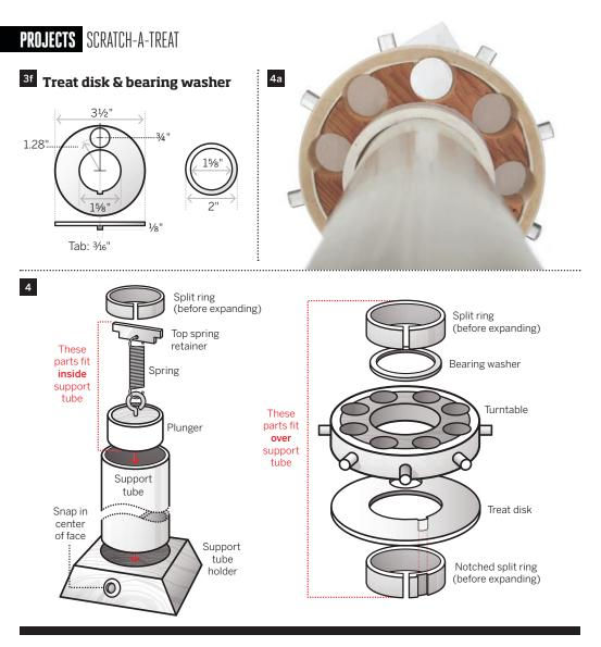
**3e.** After the turntable is completed, sand the large center hole so it rotates freely on the support tube.
